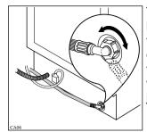
To make this easier, the hose itself may be turned to the left or the right. In either case, be sure to incorporate the strainer (A) supplied with the machine into the joint. See picture.
